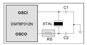
Fig. 5-30 Crystal/Resonator Circuit
